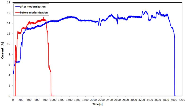
Fig. 9. Load current of the microturbine (before and after its modernization) vs. time
