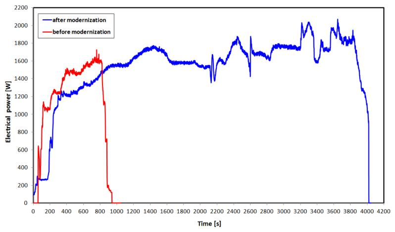
Fig. 6. Electrical power generated by the microturbine (before and after its modernization) vs. time
