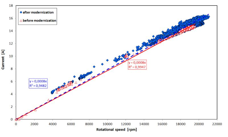
Fig. 11. Load current of the microturbine (before and after its modernization) vs. rotational speed
