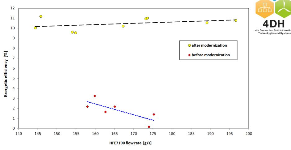
**Fig. 19.** Exergetic efficiency vs. HFE7100 flow rate (before and after the microturbine modernization)
