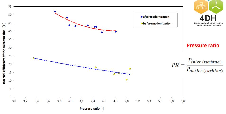
Fig. 13. Internal efficiency of the microturbine (before and after its modernization) vs. pressure ratio
