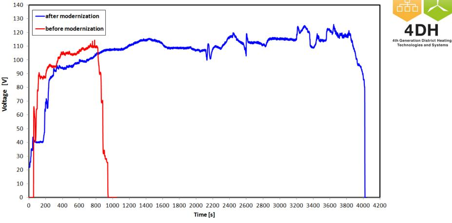
Fig. 8. Voltage generated by the microturbine (before and after its modernization) vs. time
