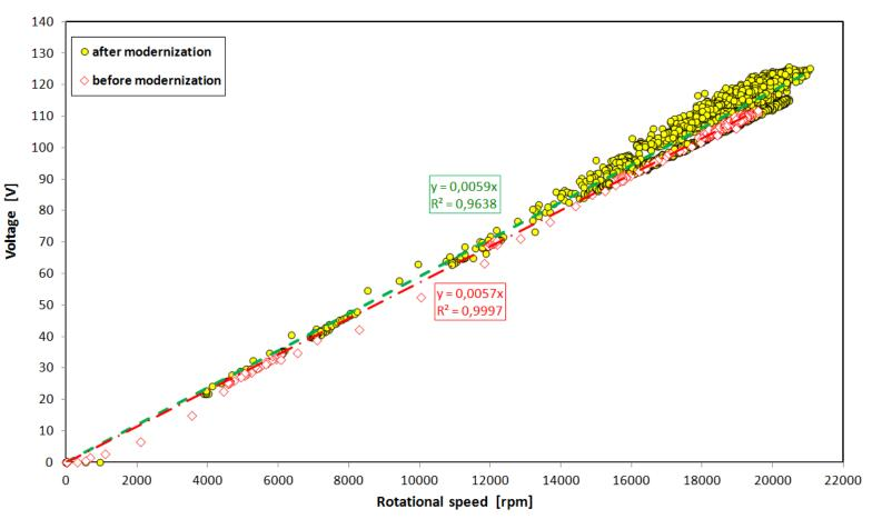
Fig. 10. Voltage generated by the microturbine (before and after its modernization) vs. rotational speed
