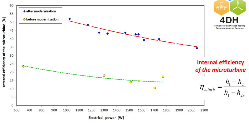
Fig. 12. Internal efficiency of the microturbine (before and after its modernization) vs. electrical power
