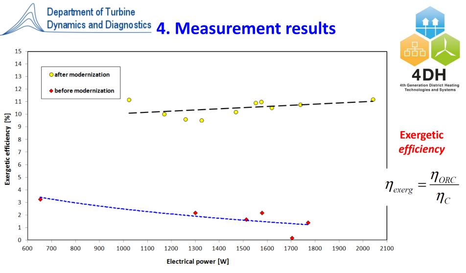
**Fig. 18.** Exergetic efficiency vs. electrical power generated by the microturbine (before and after its modernization)
