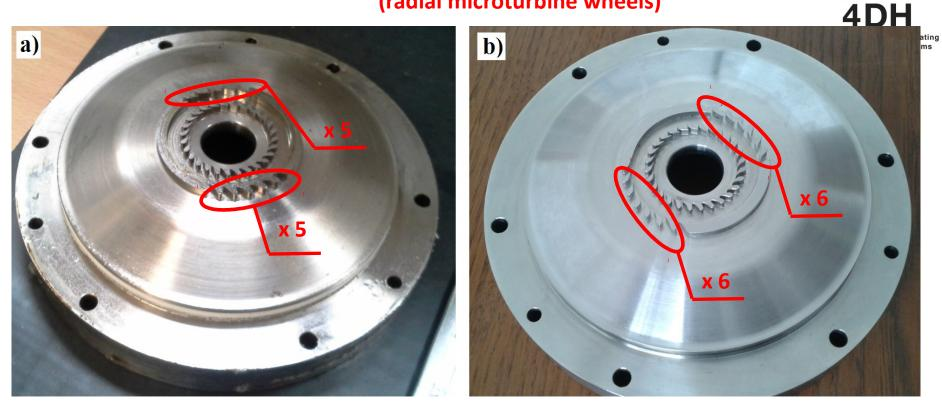
Fig. 4. Photo of the microturbine wheel: a) before and b) after the modernization
