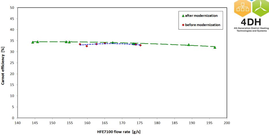
**Fig. 17.** Carnot efficiency vs. HFE7100 flow rate (before and after the microturbine modernization)
