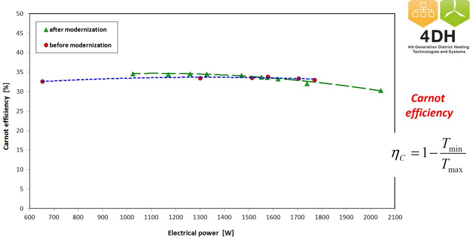
**Fig. 16.** Carnot efficiency vs. electrical power generated by the microturbine (before and after its modernization)
