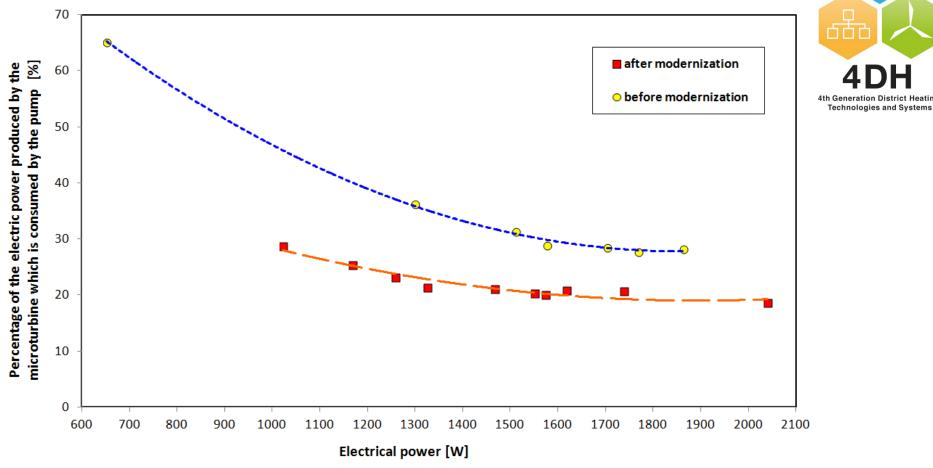
**Fig. 20.** Percentage of the electric power produced by the radial microturbine which is consumed by the pump vs. electrical power (before and after the microturbine modernization)
