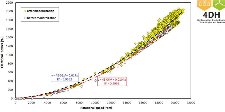
**Fig. 7.** Electrical power generated by the microturbine (before and after its modernization) vs. rotational speed
