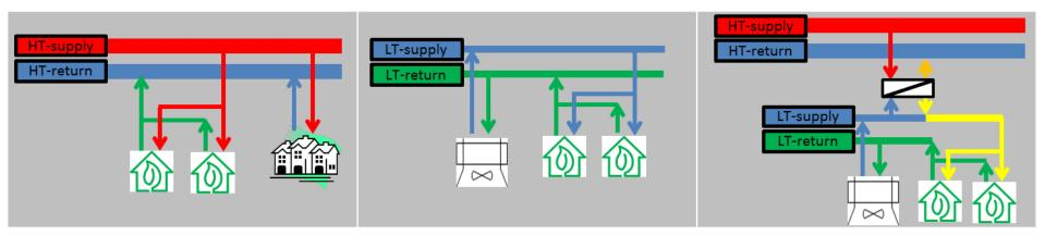
Supply temperature 90°C constant Supply temperature 49 °C constant
